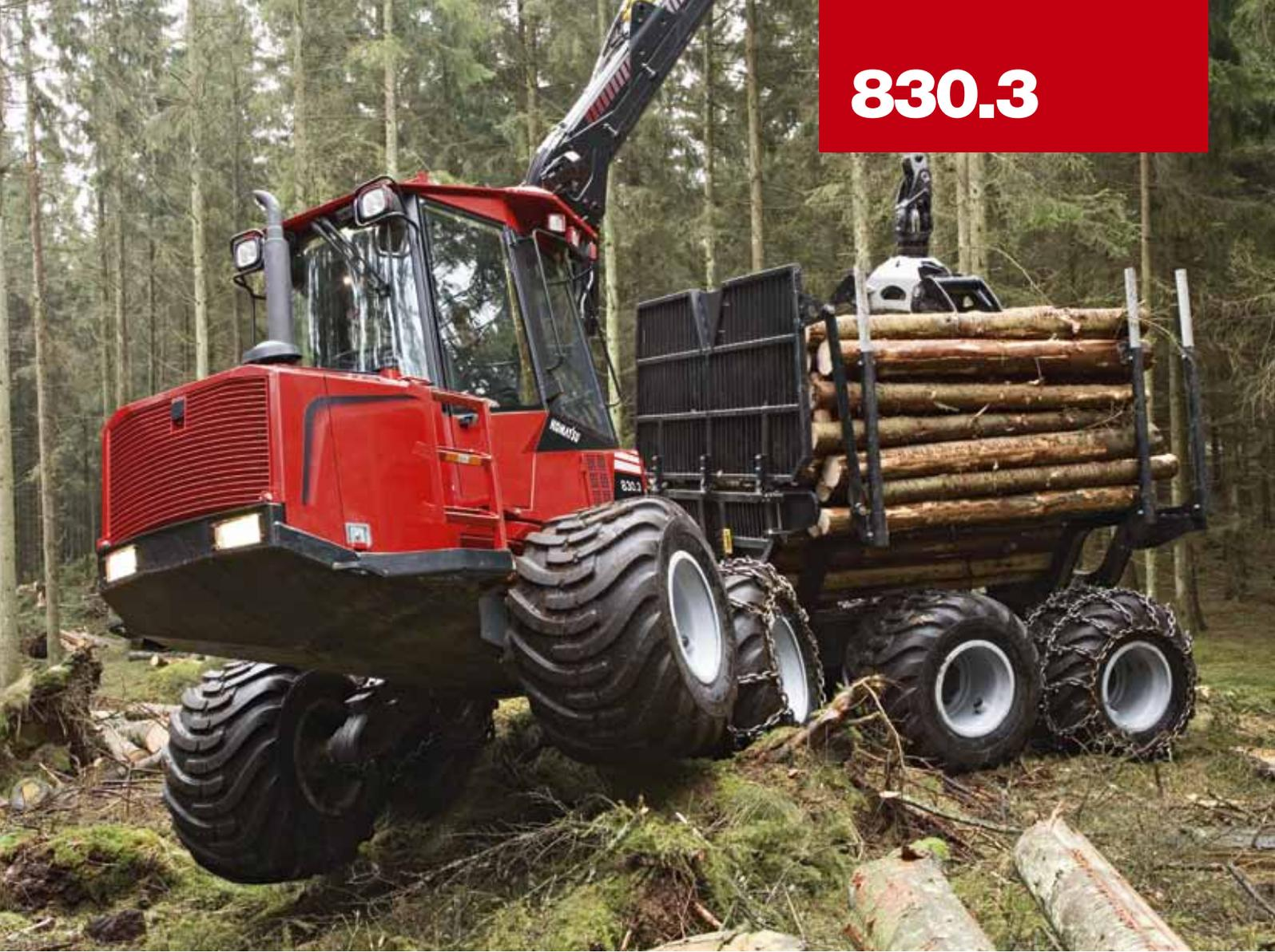
delivers ten percent more torque providing a full 600 Nm (440 lb-ft). This also applies to the already fast and nimble loader, with the lifting force increased from 67 to 74 kNm (49,400 to 54,600 lb-ft).
