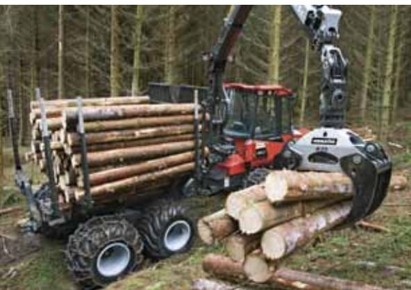
Fast and nimble thinning loader with an efficient workflow. Specially developed for the 830.3 with very good loader geometry and a lifting torque increased to 74 kNm (54,600 lb-ft).
